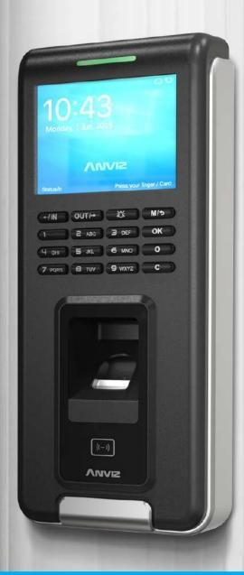
T60 pro is the new generation professional access control reader with new big 2.8" LCD screen, Liunx 1GHZ fast processor, T60pro also provides various of communication interfaces such as WIFI, POE, TCP/IP and an optional 4G function. The webserver function ensures an easily management to the device. Also 2 Relays out, Wiegand in/out functions are the standard access control interfaces. A standard EM card reader and an optional Mifare card reader is equipped onto T60 pro.
